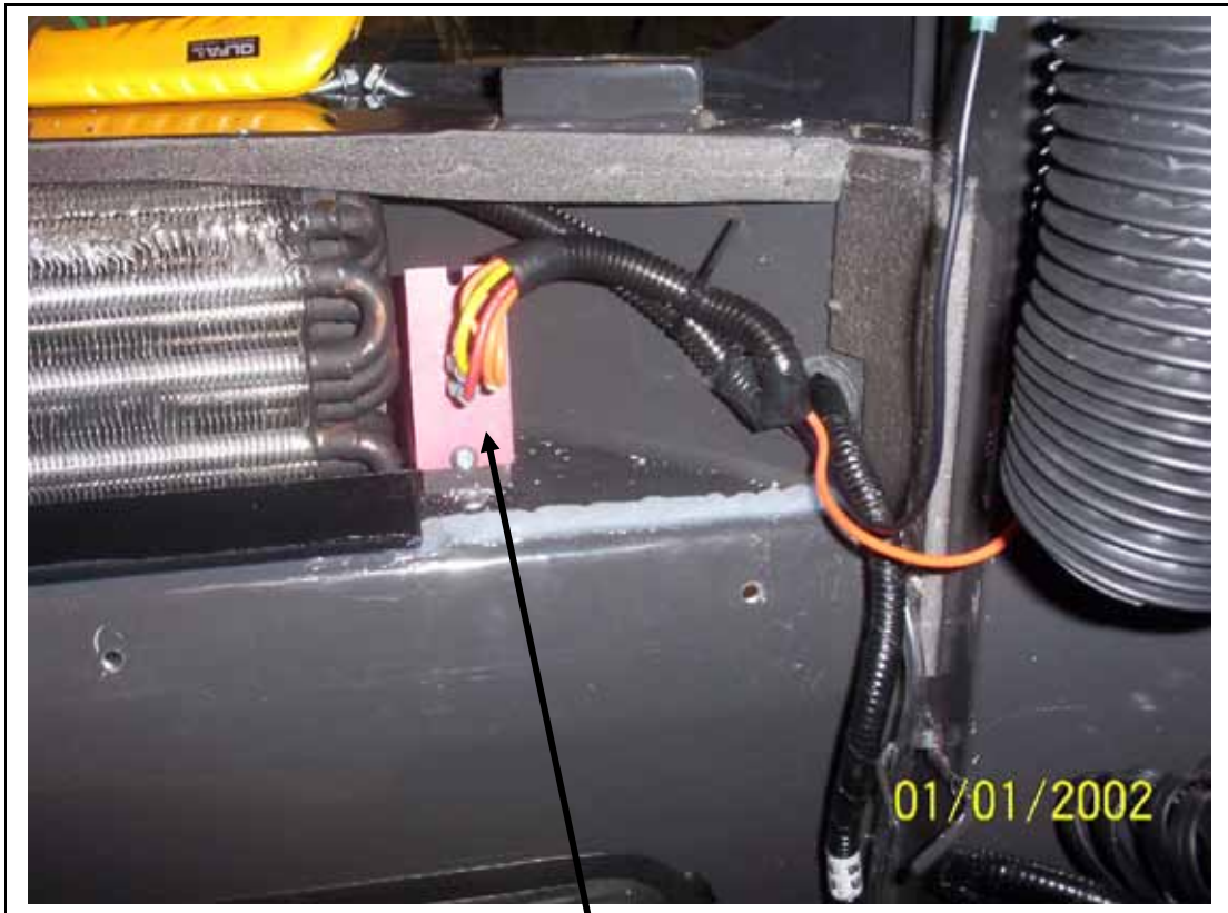
12v resistor with fan wires.
