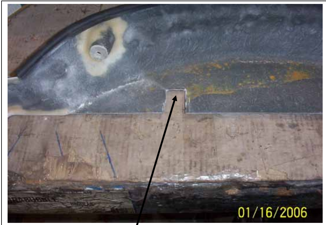
Notch out plastic cover to clear the hoses coming out of the evaporator.
