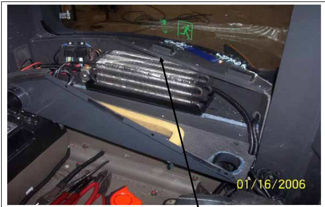
Evaporator cover open to run wiring.
