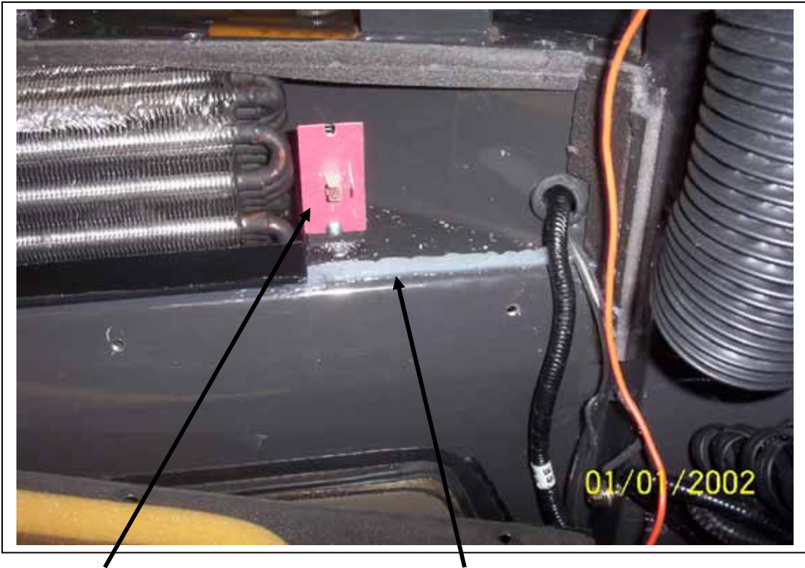
Mount resistor and bracket using two #10x3/4 self tapping screws.
