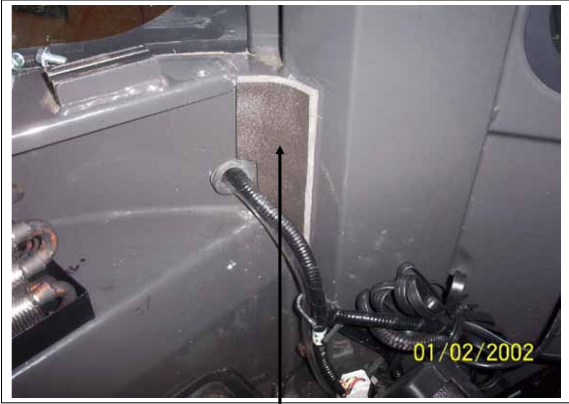
Self adhesive foam to seal evaporator box.
