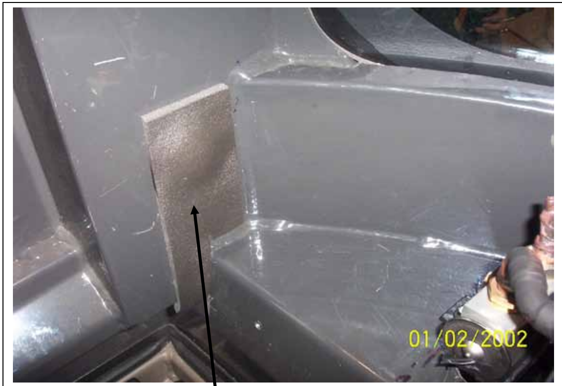
Notch and install self adhesive foam as shown.
