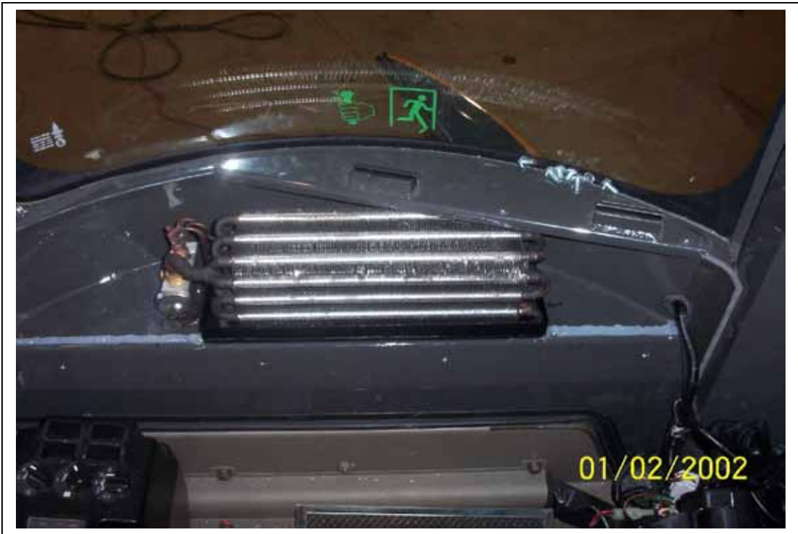
Install evaporator coil and drain pan.
