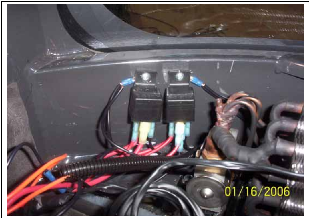
Mount two 12v relays ½" from top edge of back panel. **NOTE: All grounds
