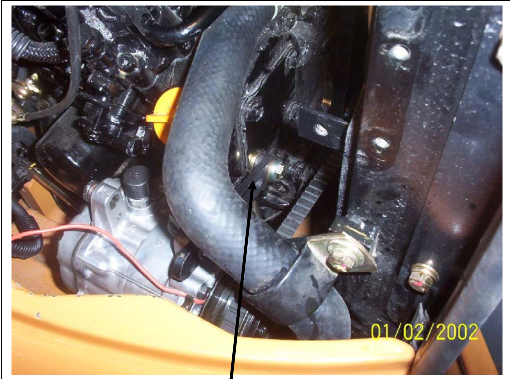
Tightener bracket installed. 3/8" spacer and M8 bolt supplied in kit.
